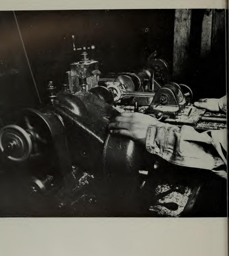
The lathe used in the above picture is identical with the one shown in Picture 21, however it is used for finishing babbitt bearings to special undersizes as ordered by the customer. About 20% of the connecting rods rebabbitted by the plaintiff are bored to special undersizes for the reason that the crankshafts of the automobiles in which they are to be placed have been reground in order to correct for the wear which has resulted from long operation.
